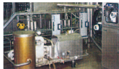
Two Ultracac 2000 dryers installed in a bottling plant
