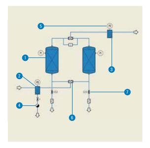
The time-controlled adsorption dryer without capacity control operates with a predetermined cycle time for which the dryers is designed, irrespective whether the desiccant might be loaded to the maximum. The dryer's requirement for regeneration air (energy consumption of compressed air) therewith remains constant.
