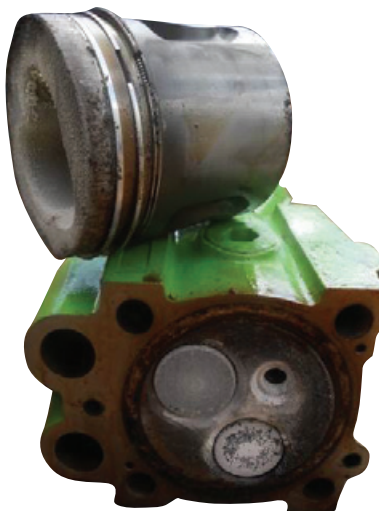
Silica deposits on a head & valves causing a collision between valves and piston crown
