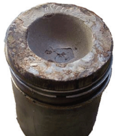
A piston coated in silica deposits
