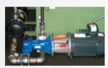
All TURBO-AIR compressors feature a self-contained, low pressure lubrication system.
